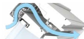
PASSIVE VENT-For controllable passive ventilation when you want it.
